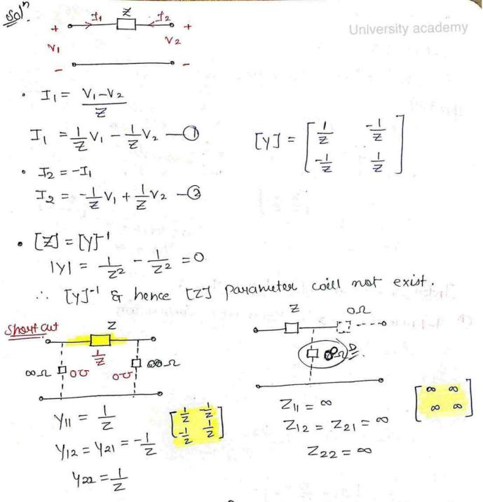
Q. Calculate the Z & y Parameters of below griven nlw.
